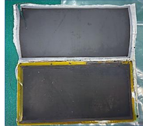
Figure 2. Disassembled cell after the test.
